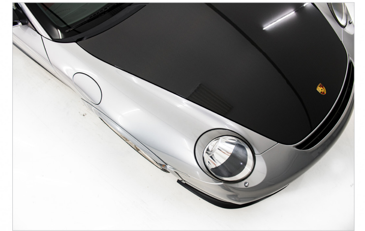
The 997 GT2 RS spoiler is sculpted with air intakes and is a more elegant piece than the 911 RSR-mimicking rear wing of the 997 GT3 RS 4.0. Both of the 997s have carbon-fiber hoods and front fenders.
