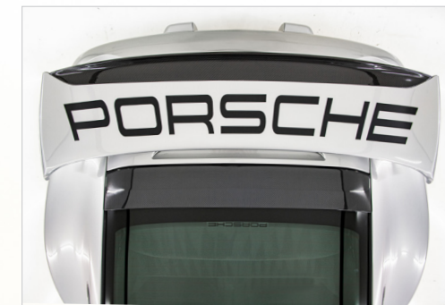
The 997 GT2 RS spoiler is sculpted with air intakes and is a more elegant piece than the 911 RSR-mimicking rear wing of the 997 GT3 RS 4.0. Both of the 997s have carbon-fiber hoods and front fenders.
