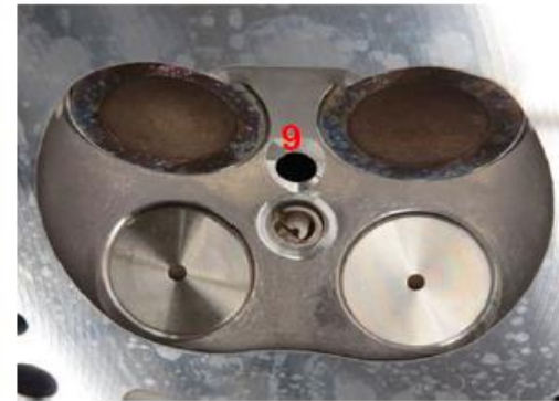
2_07_16 Injector position 8 7-hole injector 9 Central injector position
