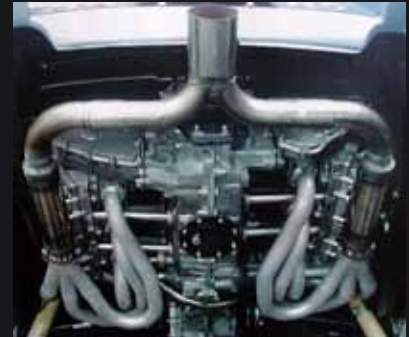
Mandrel Bent 911 RSR Headers with Silencer / Stinger Exhaust
